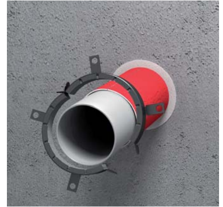
3. Select the correct collar size (in problematic built-in situations the use of an oversized collar is permitted up to max. 3 sizes bigger)
