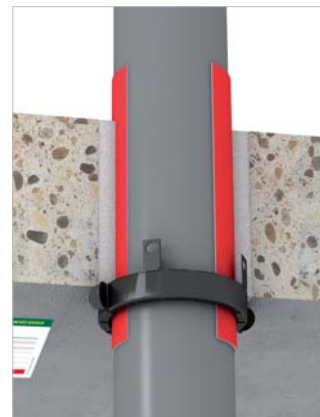
■ Fixing tabs mortared (90° reversed)
